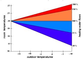
The priority task is to assure an adequate flow for the last heating elements in the system, which are deprived of warmth the most. On the other hand, one must ensure that the flow surplus does not cause overheating in nearer rooms. Specifically every 1°C results in higher costs for heating, +8% in central Europe or +12% in the case of southern Europe.
